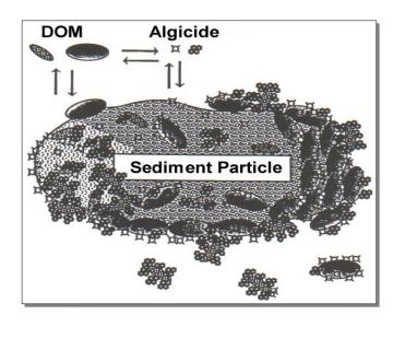
**Figure A** *(Left)*. A conceptual model of a sediment particle where different 'molecules' of dissolved organic matter (DOM) form a coating on the inorganic particle with the subsequent binding of organic algicides, mainly to the organic coating.
